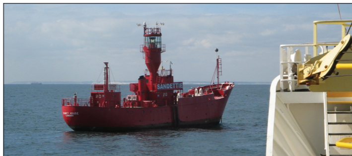
Patricia stands by to recover crew and technical personnel following a routine visit to the Sandettie light vessel on the Sandettie Bank located to the north of Calais in the Strait of Dover. Light vessels are unmanned, have no engine and are powered by solar panels.
